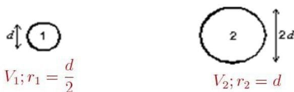
$$q_1 + q_2 = Q \Rightarrow q_1 + 2q_1 = Q \Rightarrow q_1 = \frac{Q}{3}; \quad q_2 = \frac{2Q}{3}$$
